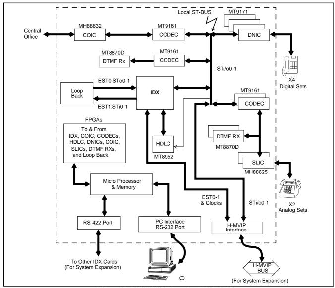
Figure 1 - MEB90812 Functional Block Diagram
